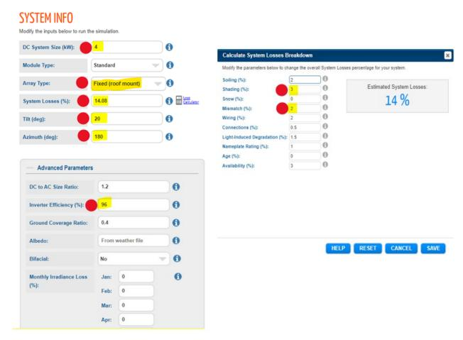
Marked fields should be filled with project-specific values for actual arrays. All other fields should be left as the default values shown
